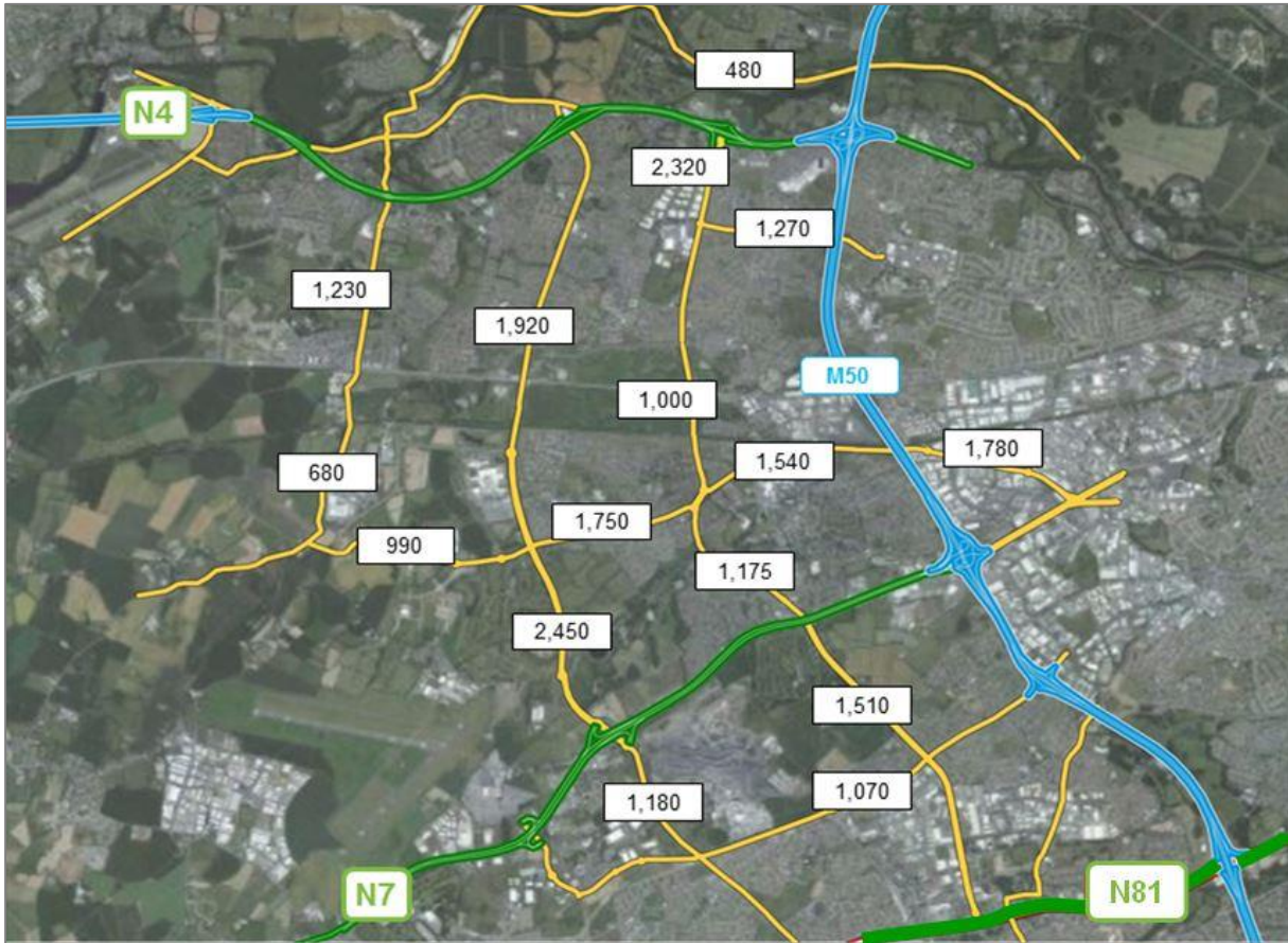
Figure 3.10: AM peak (08:00 to 09:00) two-way traffic flows on local road network Source: 2013 N4/N7 model
