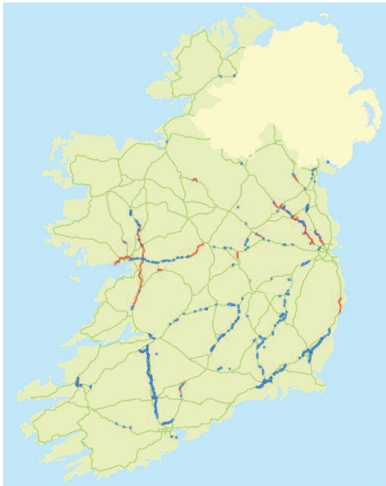
Illus. 4—Distribution of geophysical surveys carried out on the national road network. Blue dots represent isolated surveys along road schemes and red lines represent roads that have been surveyed from end to end (University of Bradford).
