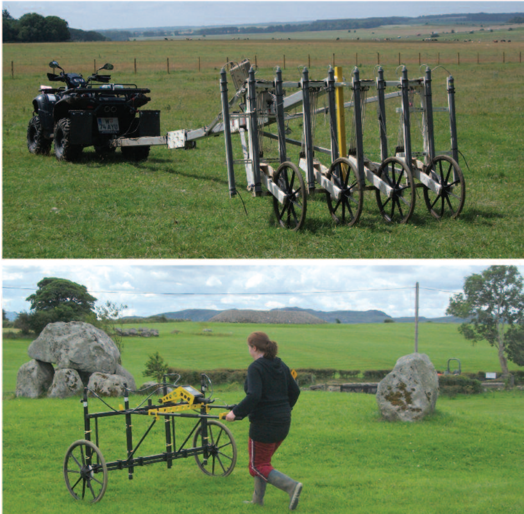
Illus. 10—The latest technology allows banks of magnetometers and/or other instruments to be used simultaneously, mounted on a wheeled array. Top: large arrays also incorporate a GPS for enhanced positional accuracy and, for larger landscapes (such as the Stonehenge environs), can be towed by an ATV to increase the speed of data collection. Bottom: for small, irregular fields, such as those at the Carrowmore megalithic cemetery, Co. Sligo, a smaller, human-propelled cart is satisfactory (University of Bradford).
