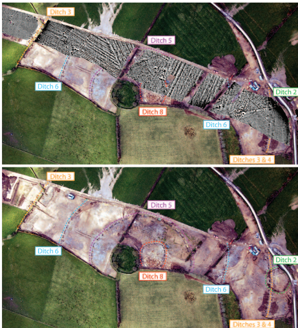
Illus. 6—Top: caesium magnetometer data from Rahally hillfort, Co. Galway (black = 2 nT (nanotesla), white = -2 nT). Bottom: post-excavation aerial view of Rahally hillfort, with major enclosing features outlined. Faint traces of Ditch 5 can be seen in the magnetometer data as a low-contrast trend beneath the strongly contrasting overprint of 19th-century cultivation furrows (after Roseveare & Roseveare 2004; photo by Markus Casey).
