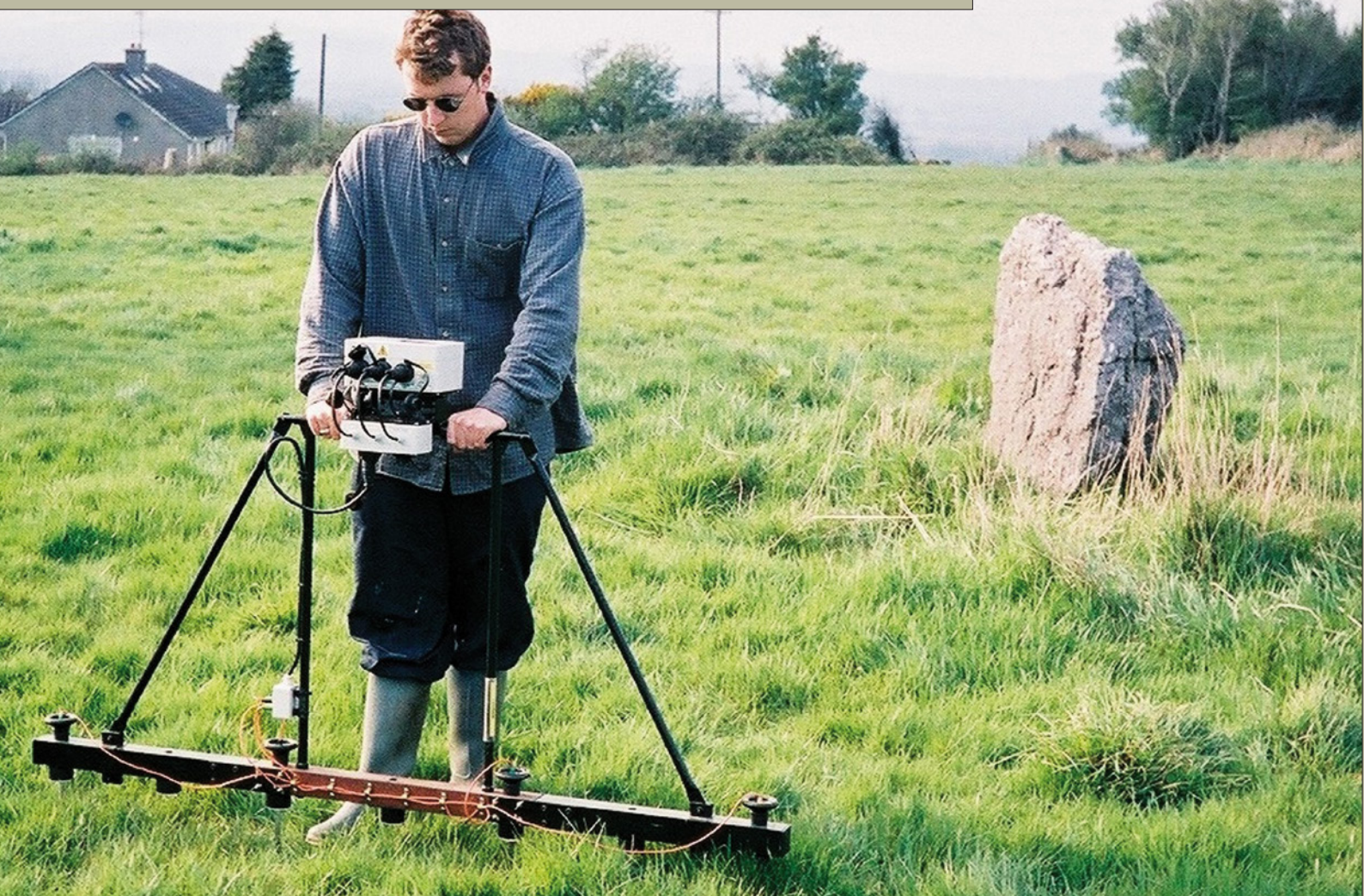
Geophysicist James Bonsall conducting an earth resistance survey at Kilmurry, Co. Kilkenny. (Photo: Earthsound Archaeological Geophysics)
