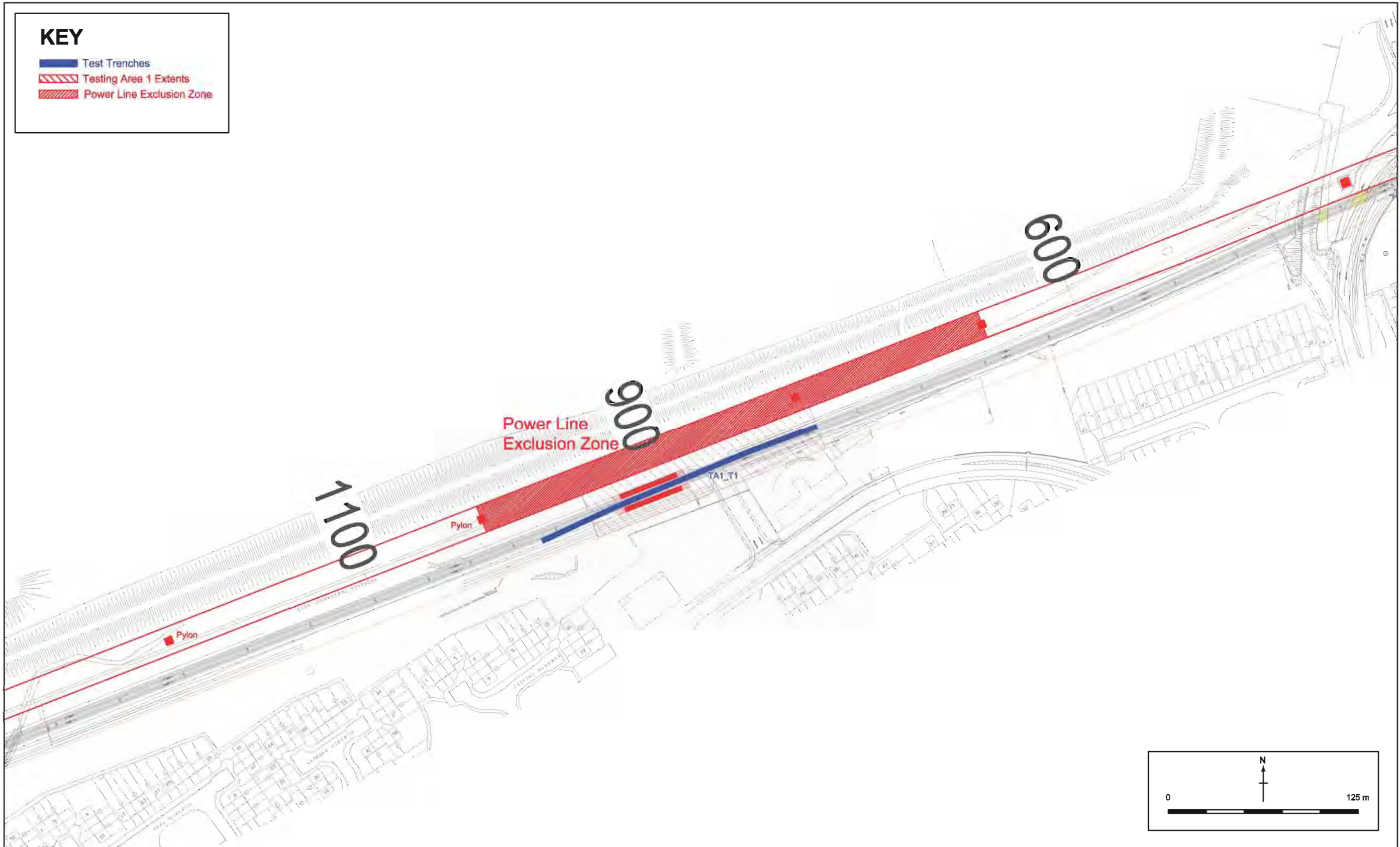
Figure 3 - Luas Line A1 Centreline Testing, Testing Area 1 Trench Layout, Fettercairn Stop.
