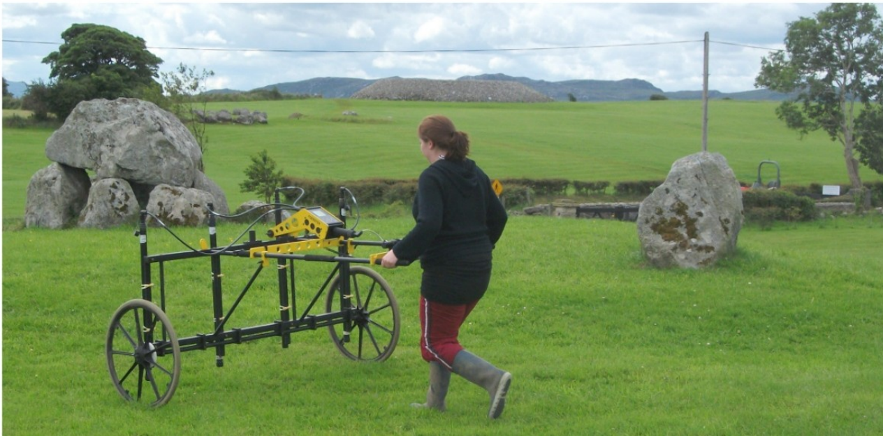
Figure 21. Cart mounted magnetometer arrays.
